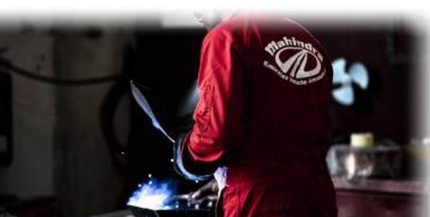
WELDING AN ARMOUR PART
